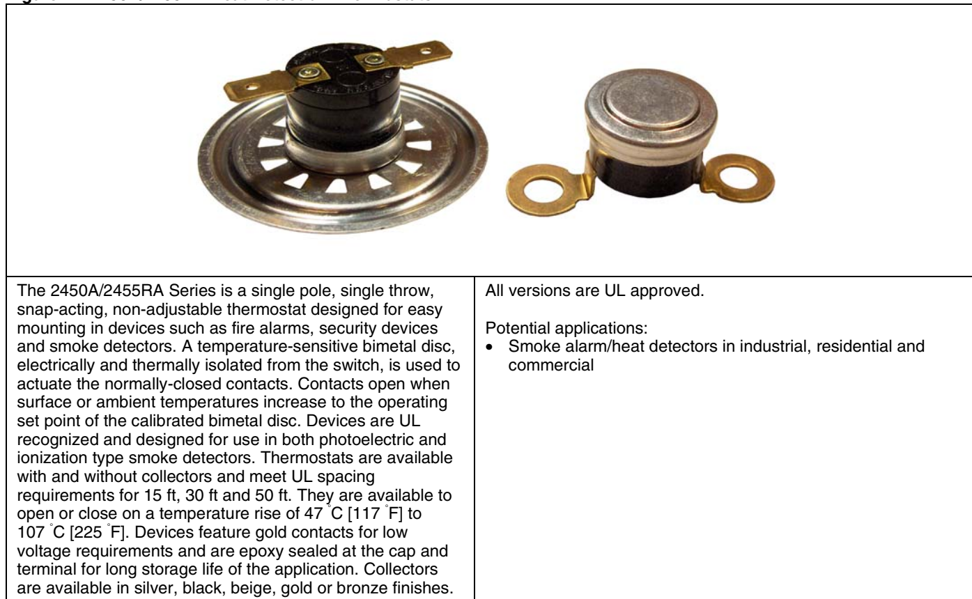
Figure 12. 2450A/2455RA Heat Detection Thermostats
